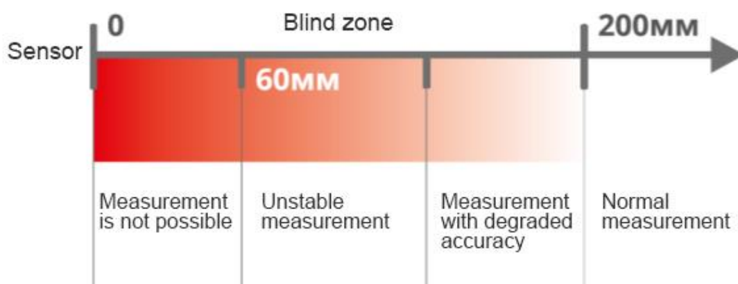
Fig. 5. Structure of the euosens MWS “blind zone”
